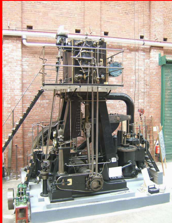
An inverted vertical compound engine built by Scott and Hodgson in 1914, named "Lily"
